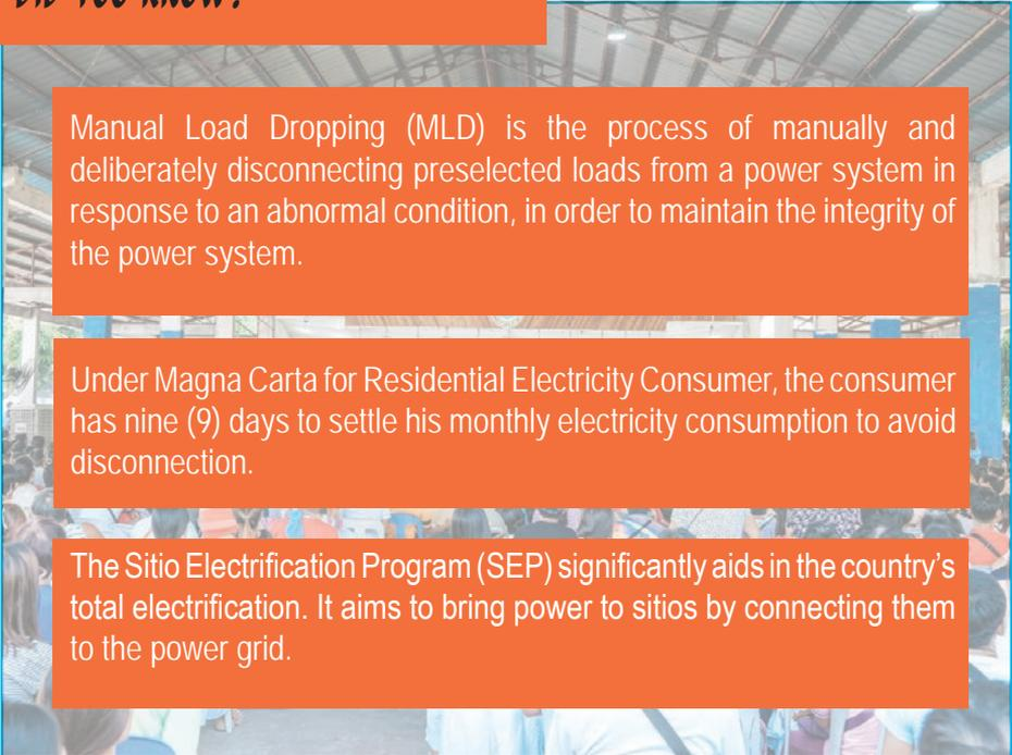
Manual Load Dropping (MLD) is the process of manually and deliberately disconnecting preselected loads from a power system in response to an abnormal condition, in order to maintain the integrity of the power system.
